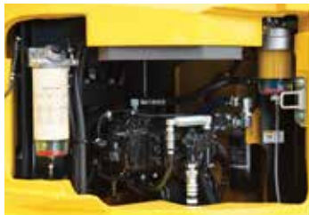
Fuel filter with built-in water-separator
