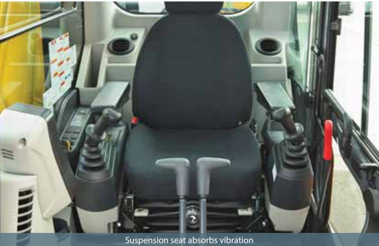
Suspension seat absorbs vibration
