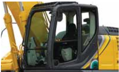
Mounting brackets for vandalism guards are standard equipment (contact your KOBELCO dealer to fit vandalism or front rock guards).
