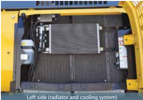
Left side (radiator and cooling system)
