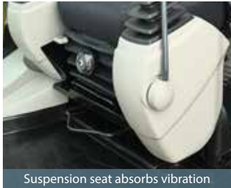
Suspension seat absorbs vibration
